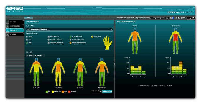
**Figure 3.4**: ErgoAnalyst Assessment page with the descriptive Hazard Profile on the left and the resulting acute and cumulative Risk Analysis Profiles presented on the right.
